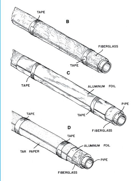
Figure 87. To Correct Sweating Pipes
