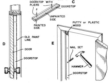
Figure 27. **Door Stop Procedure**
